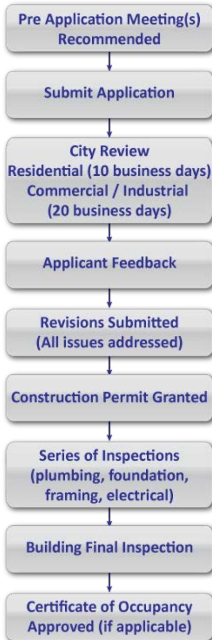
Building Inspections Flow Chart:
